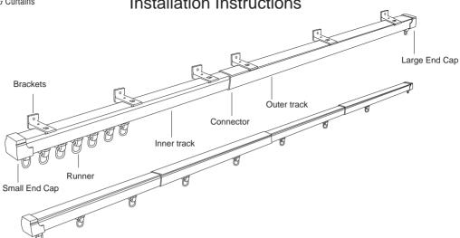
The Superglide Track can be freely extended with in the range of 110 cm - 210 cm. If the width of the window is less than 210 cm you require one track.
