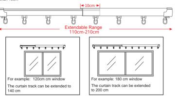
For windows greater than 200 cm, you can easily join two sets together with the joiner included in the set. You can effectively join as many tracks together to accomodate the widest of spaces.
